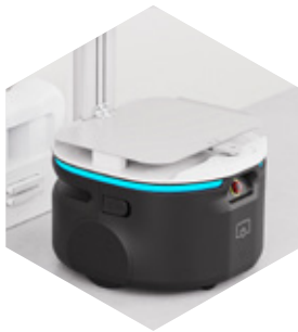
Auto-Charge: Carti returns to charging station when battery is low
